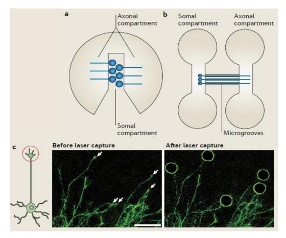
(a) The Campenot chamber made of a Teflon divider attached to a petri dish, has two compartments with distinct fluid environments. The proximal compartment contains cell bodies, dendrites and proximal axons, whereas the distal compartment contains distal axons. Typically, the distal compartment is supplemented with nerve growth factor (NGF), which promotes the growth of peripheral sensory and sympathetic neurons.
