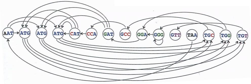
**Overlap graph problem** To generalise the construction of the graph, we form a node for each k-mer in Patterns and connect the k-mers by a direct edge if the suffix is equal to the prefix => **overlap graph**
