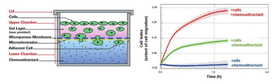
As cells move from the upper chamber towards chemoattractant in the lower chamber, they pass through a membrane containing 8  $\mu$ m pores and then adhere to gold impedance microelectrodes. The resultant **change in impedance signal perfectly correlates with the number of cells** attached to these electrodes, enabling collection of highly reproducible data over time ranges spanning from minutes to days.
