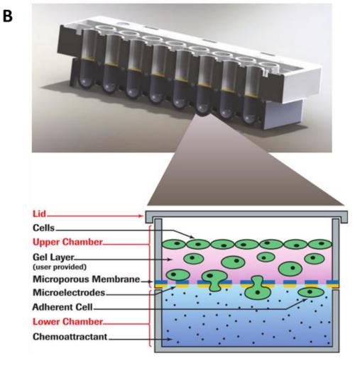
The figure illustrates the upper and lower chambers for a single well. The bottom surface of the upper chamber is composed of a microporous membrane that cells can migrate through. Gold electrodes on the underside of this membrane detect the presence of adherent cells.
