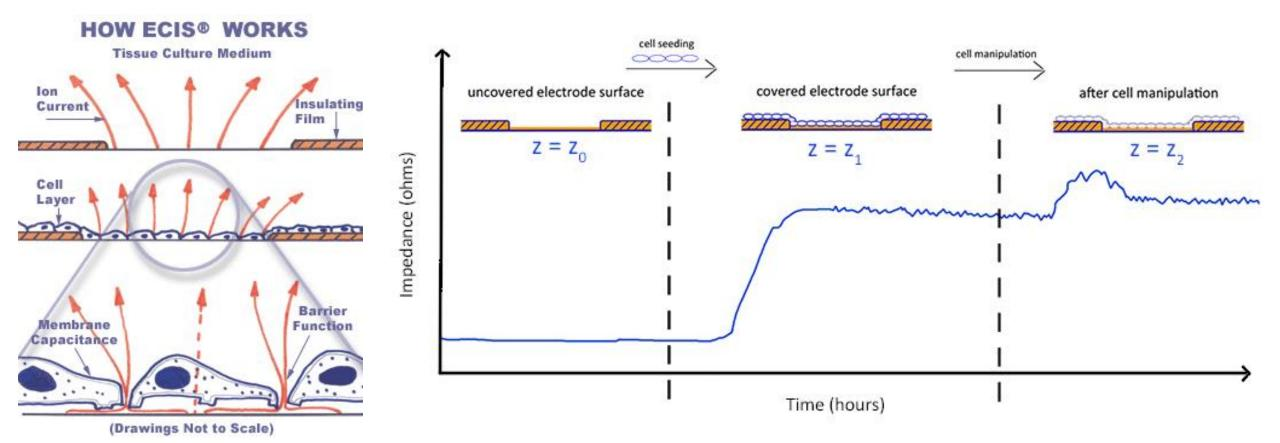
When cells attach to the electrodes, they act as insulators increasing the impedance. As cells grow and cover the electrodes, the current is impeded in a manner related to the number of cells covering the electrode, the morphology of the cells and the nature of the cell attachment.
