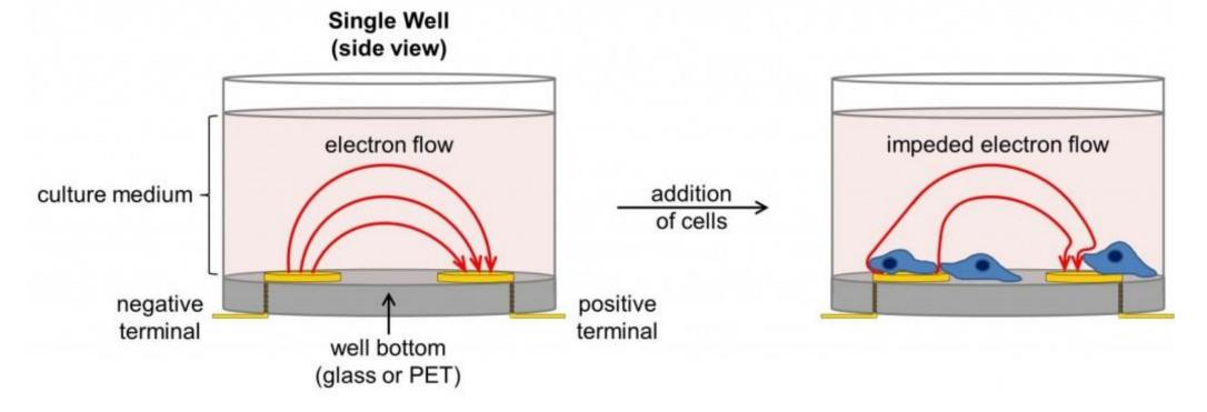
Set of gold microelectrodes fused to the bottom surface of a microtiter plate well.
